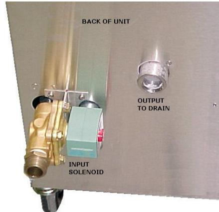
Two pumps have been installed in the unit. One pump is used for the normal draining of tank and the second pump is used with the overflow drain during the cascading rinse. On the outside of the console you will find a  $\frac{3}{4}$ " NPT bulkhead coupling which extends through the back of the cabinet. This fitting comes from the internal pumps and must be adapted to your drain plumbing using  $\frac{3}{4}$ " ID or larger tubing.
